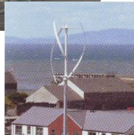
Turbina QR5 (“Quiet Revolution”) 6kW, 3=2m, L=5m (UK)
