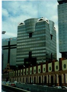
Fig. 35: A "Post-Modern" office tower in Lisbon, using tinted-glass facades, a high glazing ratio, equal in all facades, and high building depth. The glazing ratio is approximately 50%, when the recommended by the LT method 3.0 for this situation is 30 to 40% (Baker, 1994).
