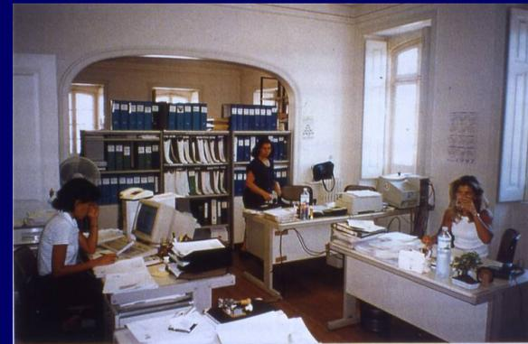
A cellular room in a typical naturally ventilated office in Lisbon, during summer. The use of building environmental controls such as fans, open windows and doors for ventilation cooling can be observed. Occupant behaviour to feel cooler during the hot day can also be observed, such as drinking cold water and wearing light clothing.
