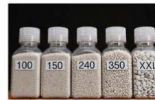
Different size fertilizer pills manufactured using Ostara's Nutrient Recovery Technologies
